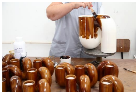
STEP 9: APPLYING VARNISH WITH A BRUSH
