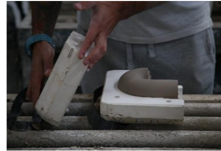
STEP 2: REMOVE FROM MOULD
