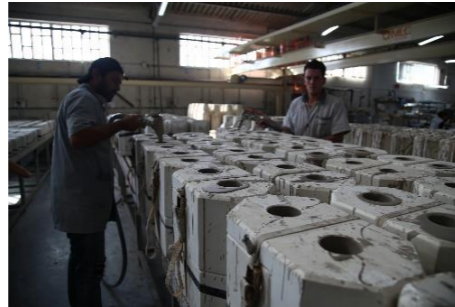
STEP 1: POUR THE LIQUID CERAMIC INTO THE MOULD
