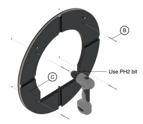
Mark the placement of the four screw holes for mounting the backplate on the wall.
