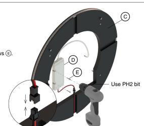
We recommend connecting the transformer directly to the main power supply placed behind the mirror as illustrated.
